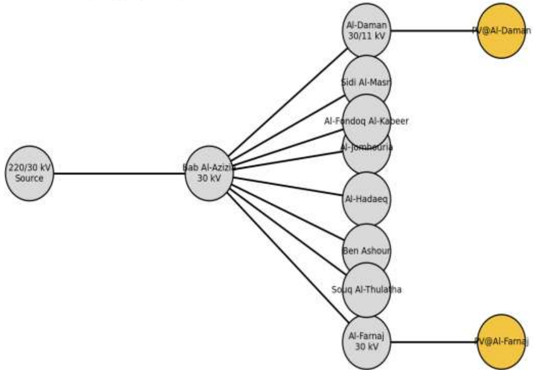
Figure. 3. MATLAB-style graph representation of the Bab Al-Azizia 30-kV network and PV support locations.
